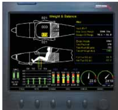
Advanced Flight's engine monitor can be displayed on an EFIS screen (left). A weight-and-balance screen helps loading (right).
