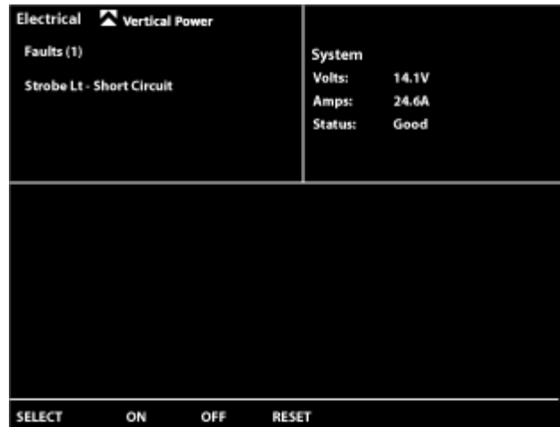
Screen showing basic status and faults.
