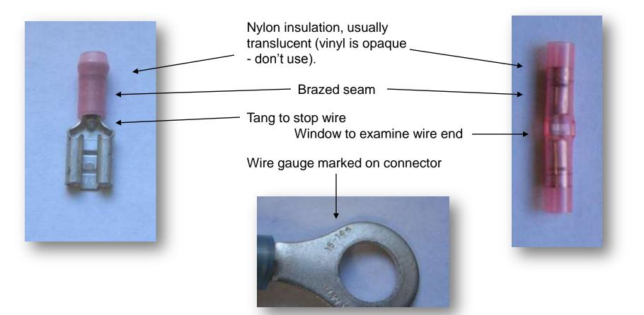
High-quality connectors have the wire gauge stamped on the metal, and the insulation is translucent (nylon)
