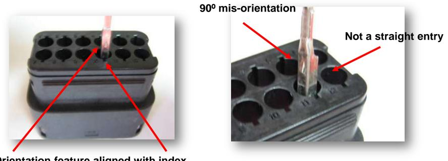
Orientation feature aligned with index
