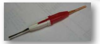
Standard d-sub tool is red/white. High density d-sub tool is green/white.
