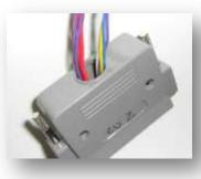
Wires can vibrate within the connector housing
